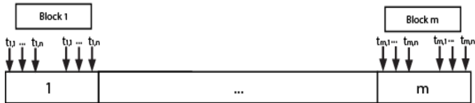
Figure 3.4: Threads in thread block read data in sections
